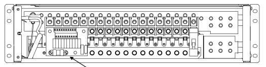
Mounting Position for First GMT Assembly When Factory-Installed
